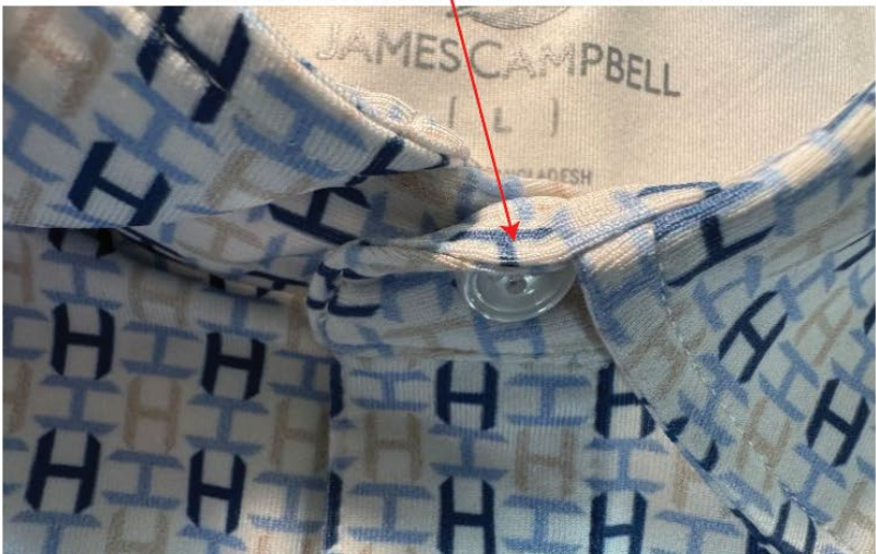
Collarband rolls down at CF - improve construction
