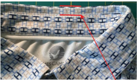
Collar roll is at band seam should be max of 1/4". Sample roll measures 1/2" and collar does not cover collar band seam in back.
