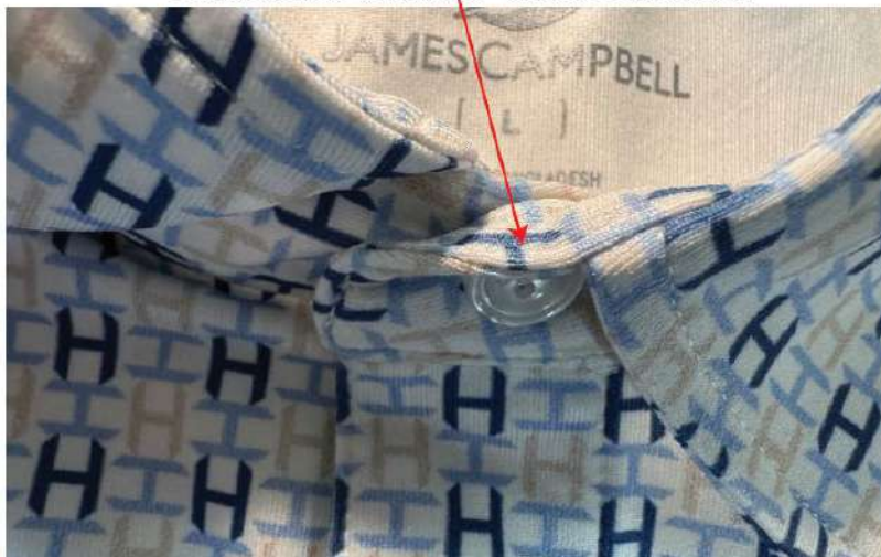
Collarband rolls down at CF - improve construction
